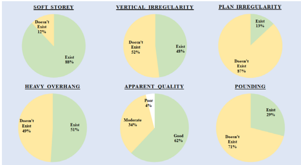
Figure 3. Distribution of various vulnerability parameters present in surveyed buildings.
