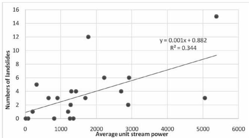
Figure 9. Relationship between exposures/landslides and average unit stream power.
