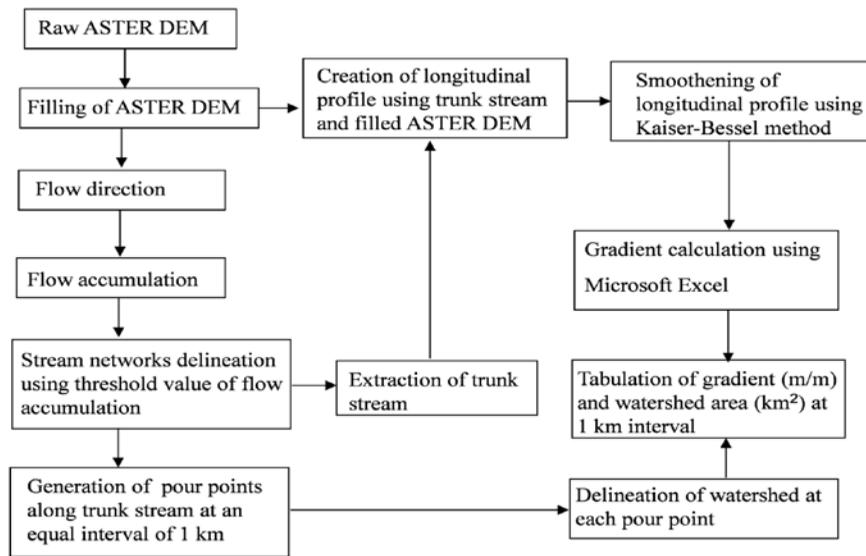
**Figure 3.** Flow chart depicting: a) procedures for delineation of the watershed, b) creation of the longitudinal profile, c) its smoothing and d) slope estimation at an equal interval of 1 km.
