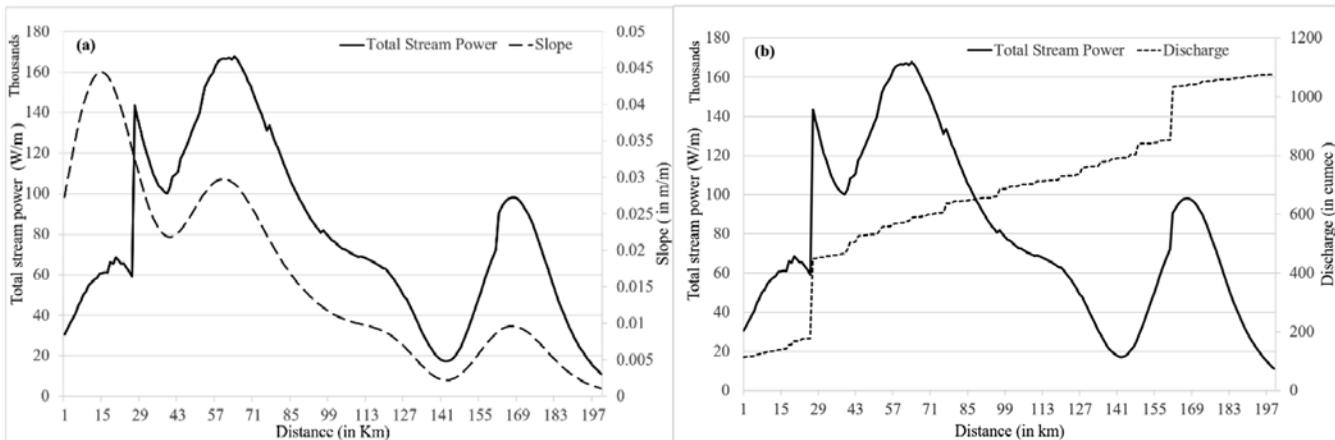
**Figure 5.** Relationship between (a) total stream power and slope and (b) total stream power and discharge in the Bhagirathi River.
