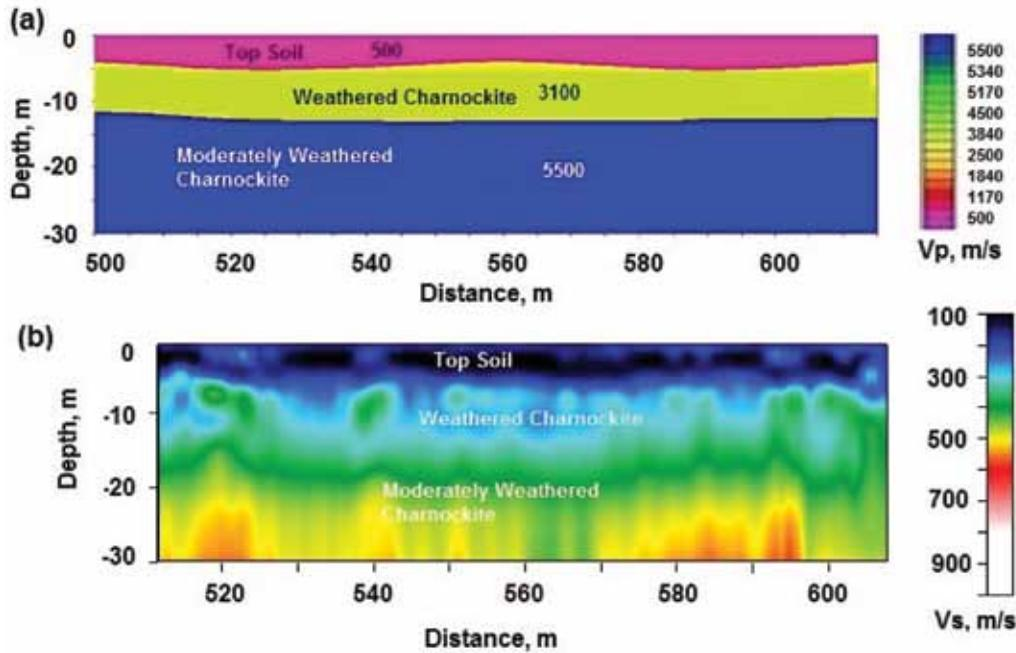
Figure 2. shows a) P-wave velocity depth section of profile 2, b) Shear wave velocity depth section of profile 2.
