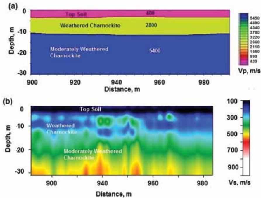
Figure 3. shows a) P-wave velocity depth section of profile 3, b) Shear wave velocity depth section of profile 3.
