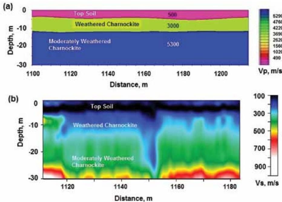
Figure 4. shows a) P-wave velocity depth section of profile 4, b) Shear wave velocity depth section of profile 4.
