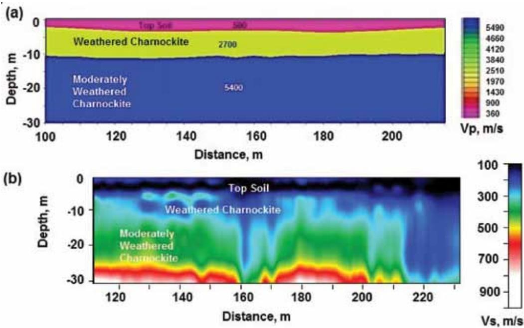
Figure 1. shows a) P-wave velocity depth section of profile 1, b) Shear wave velocity depth section of profile 1.
