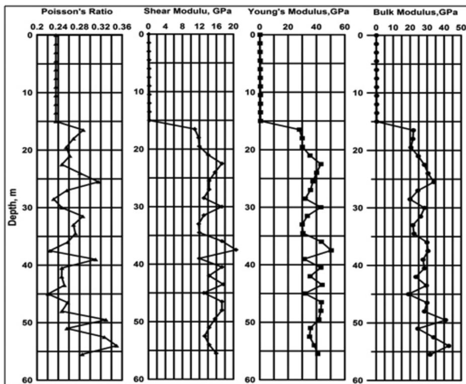
Figure 3. Shows the plot of calculated elastic moduli ((GPa: Giga Pascal)).
