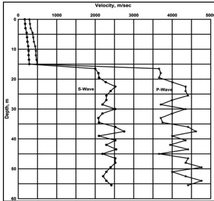
**Figure 2.** Shows the plot of calculated P & S wave velocities of the subsurface concerning depth. (m/s: meter/second).
