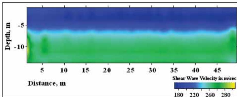
**Figure 5.** Shows the Shear wave velocity field consists of two velocity layers. It is interpreted that the soil cover and weathering cap of varying consolidation are characterized by an S-wave velocity of  $\sim 160\text{-}240$  m/s, and  $\sim 240\text{-}350$  m/s, respectively.
