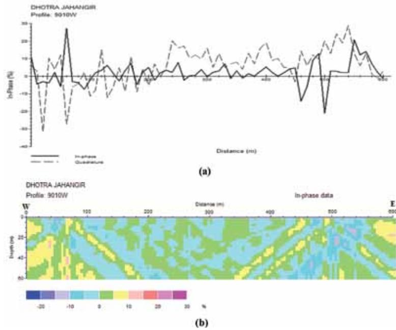
Figure 3. VLF-EM Profile 9010W (a) Real and Imaginary components (b) Pseudo-depth section.
