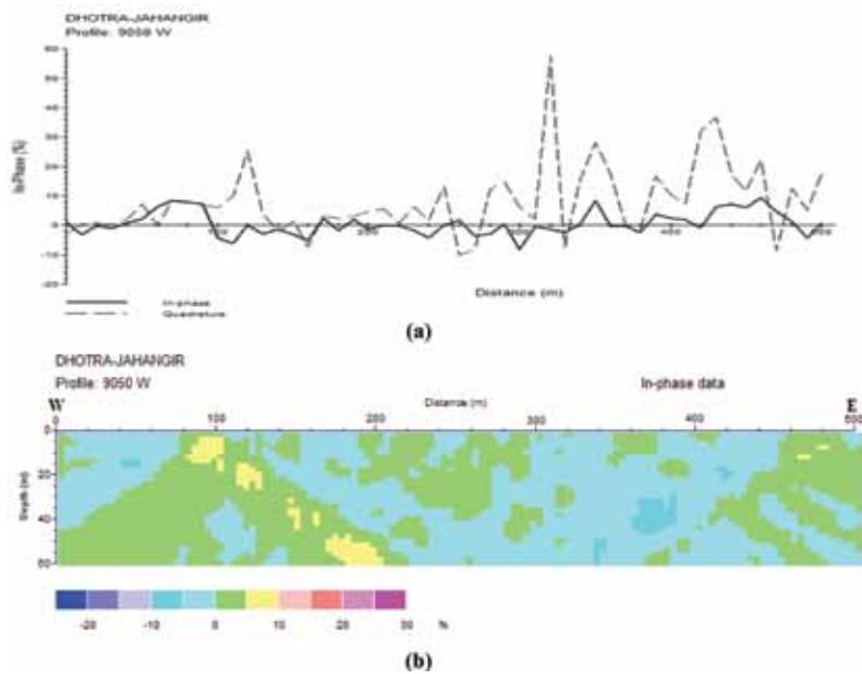
Figure 5. VLF-EM Profile 9050W (a) Real and Imaginary components (b) Pseudo-depth section.
