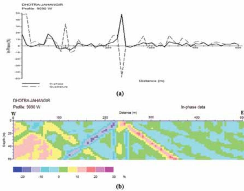
Figure 7. VLF-EM Profile 9090W (a) Real and Imaginary components (b) Pseudo-depth section
