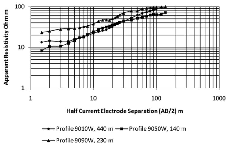
**Figure 9.** VES on profiles 9010W at 440 m, 9050W at 140 m and 9090W at 230 m observation points.
