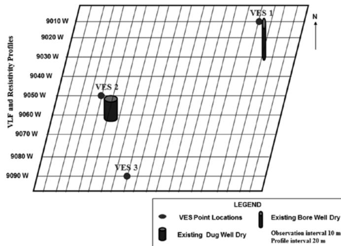
**Figure 2.** Profile Layout for VLF-EM and Resistivity Profiling surveys (not to scale)
