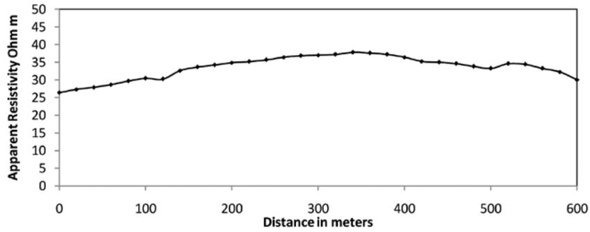
Figure 6. Gradient Resistivity Profile along P 9050W.
