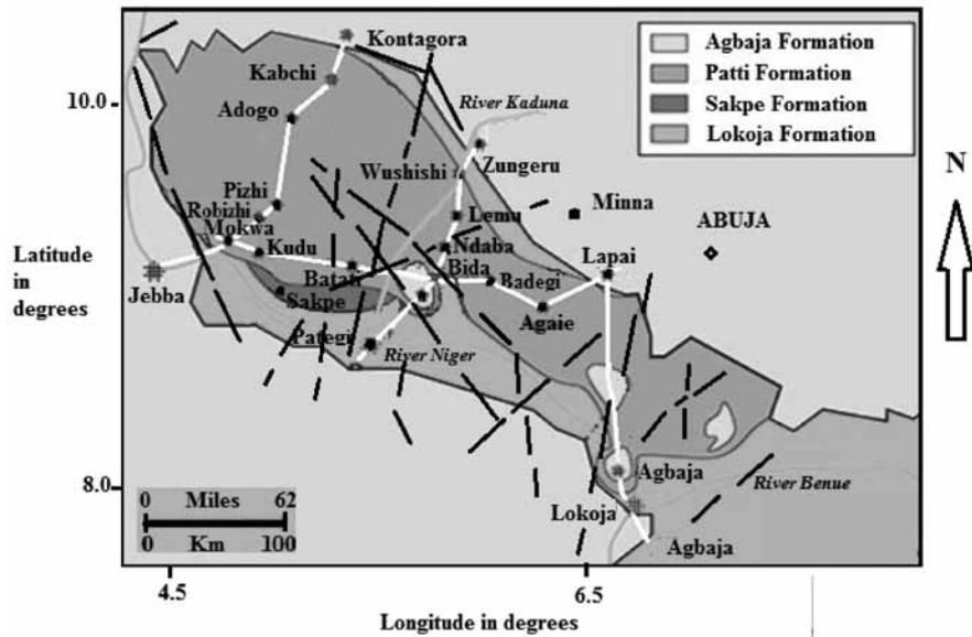
Figure 2. Geologic map of Bida basin showing stratigraphic sequence and lineaments (After NGSA, 1984; Obaje et al., 2015)
