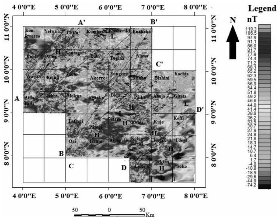
**Figure 4.** Residual Total Magnetic Intensity Map (RTMI) of entire Bida basin showing inferred lineaments (AA', BB', CC' and DD') – likely paleofracture zones. Magnetic high (H) and low (L) are also shown. A constant 33000 nT was removed as common background field.
