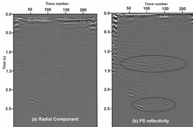
**Figure 5.** The result of deconvolution of the radial component data with the downgoing wavefield. (a) shows the radial (R) component, while (b) shows the PS reflectivity obtained as a result of deconvolution. Significant improvement in the signal resolution can be noticed in (b) at almost all times and is highlighted as dashed ovals.
