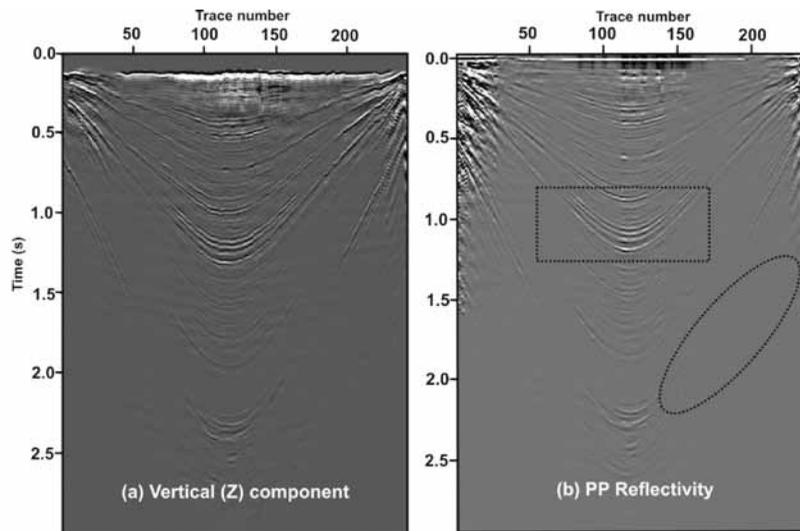
**Figure 4.** The result of deconvolution of the vertical component data with the downgoing wavefield. (a) shows the recorded vertical (Z) component, while (b) shows the PP reflectivity obtained as a result of deconvolution. Significant improvement in the signal resolution can be noticed in (b) and is highlighted as a dashed rectangle. The dashed oval in (b) shows the attenuation of the multiples and cleaner vision of the marked area compared to (a).
