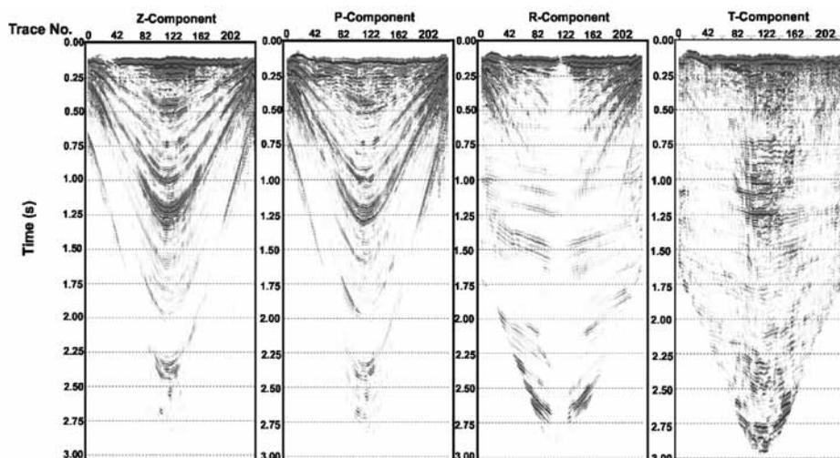
**Figure 2.** The OBS data acquired in the Mahanadi basin. The vertical (Z) component, the hydrophone (P) component data are retrieved from the instrument and can be treated as field data, while the radial (R) and the transverse (T) component of data are obtained by rotating the two orthogonal (X,Y) components from the field data, in such a way that the energy is maximum on the radial component.
