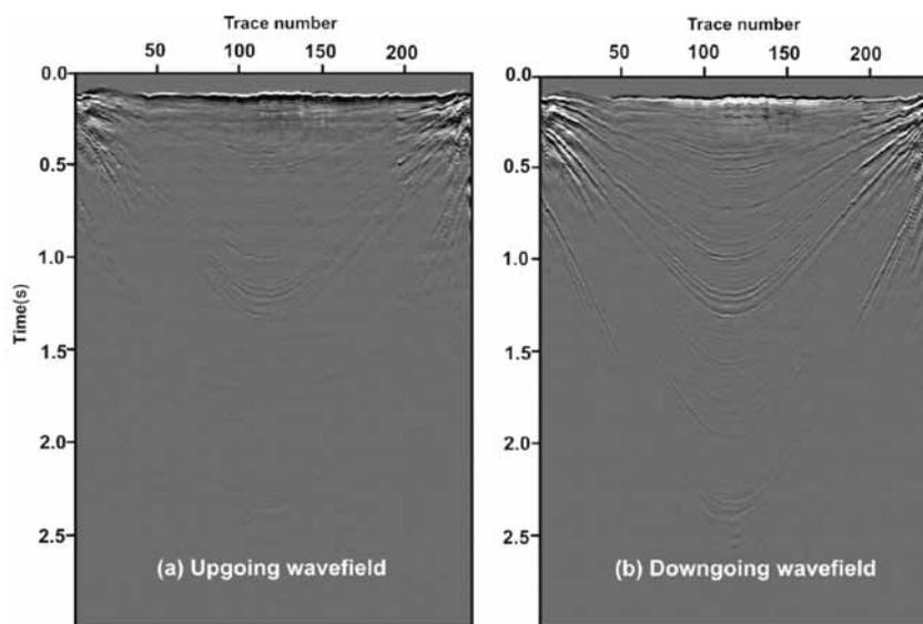
**Figure 3.** The result of the wave field decomposition. The recorded wavefield is decomposed into the (a) up-going wavefield and (b) down-going wavefield. The up-going wavefield is dominated by the shallow multiples, while the down-going wavefield shows the sharp down-going wavefield, which is later used in the deconvolution.
