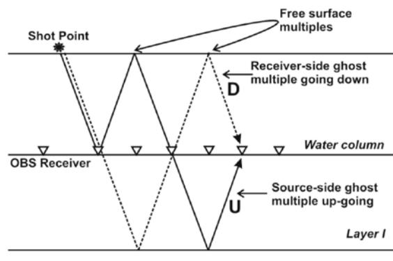
**Figure 1.** A schematic diagram showing the source-OBS configuration in a marine setting, along with the up-going and down-going waves and their travel paths.
