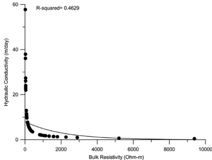
Figure 2b: Correlation plot between bulk resistivity and hydraulic conductivity ( $k$ ).
