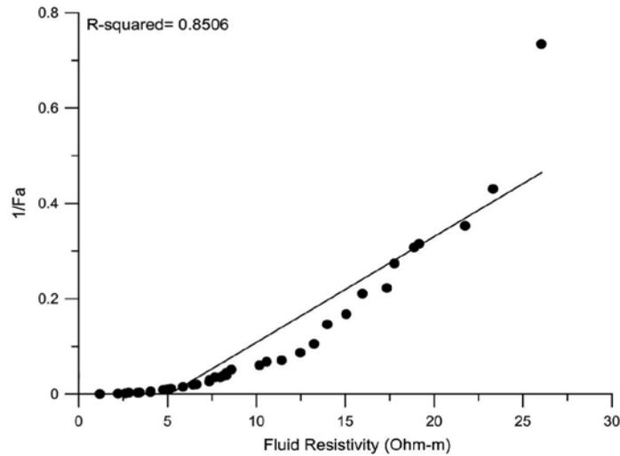
Figure 2a: Determination of the intrinsic formation factor  $F_1$  by plotting  $1/F_a$  versus fluid resistivity  $\rho_w$ .
