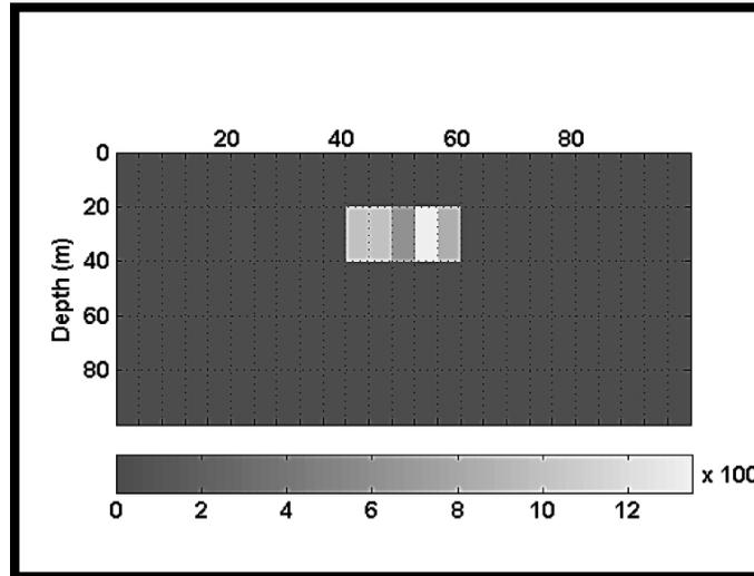
Figure 5. The result of the inverse modeling for the theoretical model (with 20% random noise).
