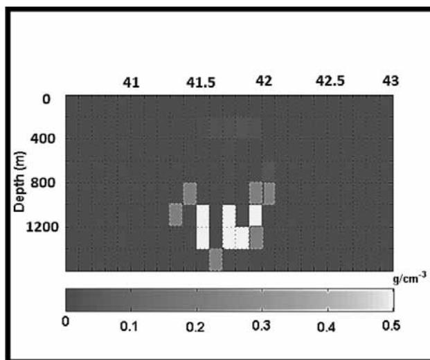
Figure 9. The result of the inverse modeling for the salt dome.
