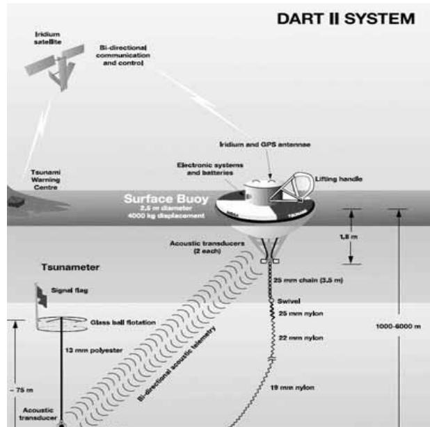
Figure 1. A schematic representation of a deep-ocean tsunami detection buoy (DART™).
